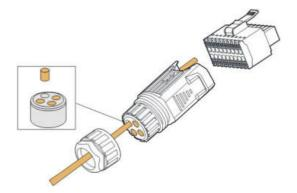
step 4 Remove the cable jacket by 7 mm-10 mm.
