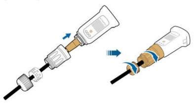
step 6 Remove the waterproof lid from the WLAN terminal and install WiNet-S.
