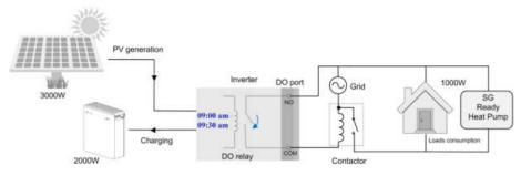
figure 8-25 DO Operation in Intelligent Mode
