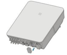
step 3 Align the Backup connector and the **BACK-UP** terminal and mate them together by hand until a "Click" is heard or felt.
