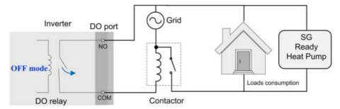
figure 8-24 DO Operation in Switch Mode
