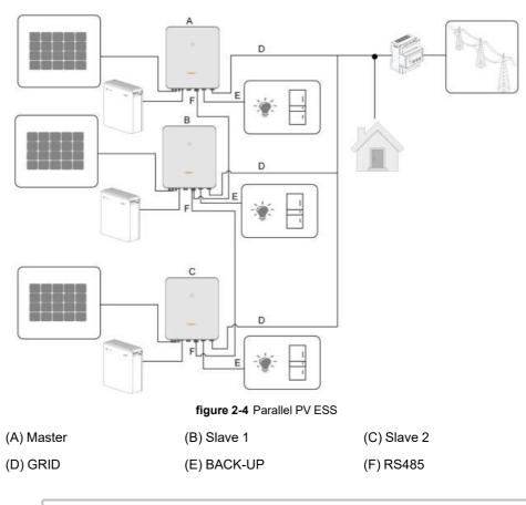
Only the inverter GRID terminal can be connected in parallel, the BACK-UP terminal and the battery terminal cannot be connected together, they should be connected to the off-grid load and the battery respectively. The Backup loads of each inverter should not exceed its nominal power.
