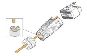
step 4 Remove the cable jacket and strip the wire insulation.
