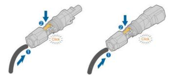
step 4 Push the insert into the sleeve and tighten the cable gland (torque 2 N·m).
