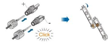
step 4 Check for polarity correctness.
