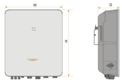
figure 2-2 Dimensions of the Inverter
