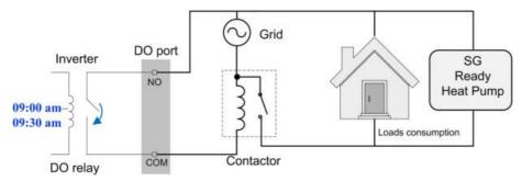
figure 8-23 DO Operation in Timing Mode
