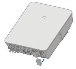
step 3 Insert the AC connector into the **GRID** terminal on the bottom of the inverter until there is an audible sound.
