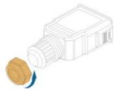
step 2 **(Optional)** Remove the inner sealing ring if the cable diameter is between 19 mm ~ 25 mm. Otherwise skip this step.
